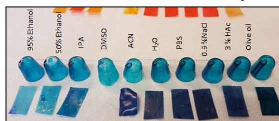
Fig. 1: Effect of different solvents on the same sample in plane and moulded form.
